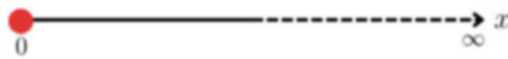
Fig. 4.1 Schematic representation of a one-dimensional semi-infinite domain with an absorbing end at x = 0 (red circle)
