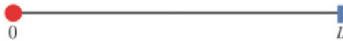
Fig. 5.7 Schematic representation of a one-dimensional domain with an absorbing point at x = 0 (red circle) and a reflecting target at x = L (blue bar)
