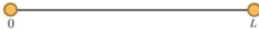
Fig. 7.7 Schematic representation of a one-dimensional domain with two partially absorbing endpoints (yellow circles), one at x = 0 and the other at x = L
